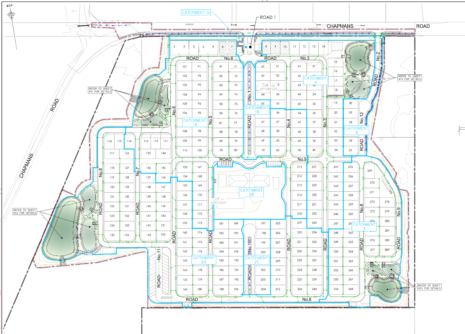
STORMWATER DETAIL PLAN SCALE 1:1000
