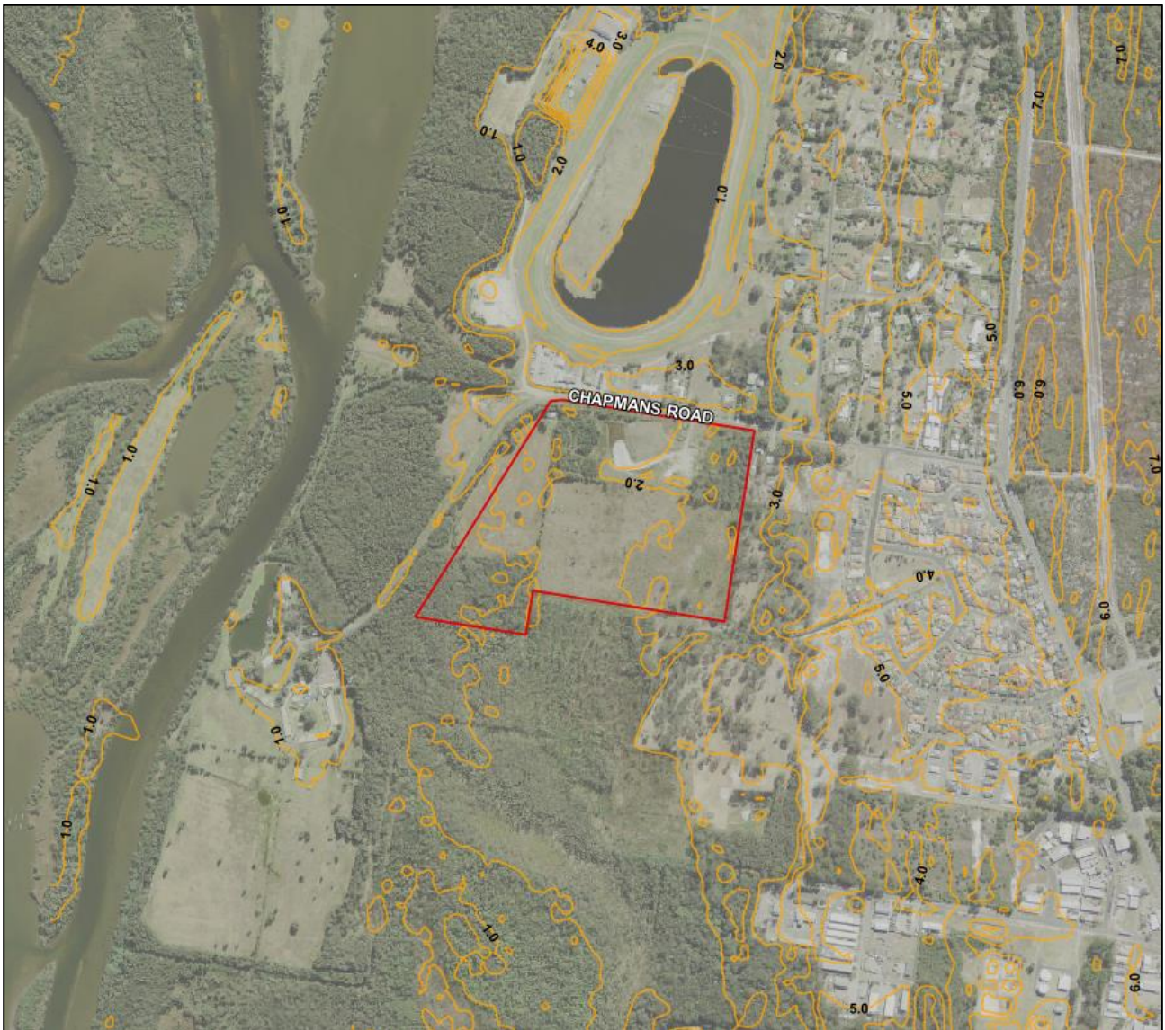
Figure 12: Pre development ground surface, 1 m contours (m AHD) imported into MODFLOW, site boundary shown in red outline
